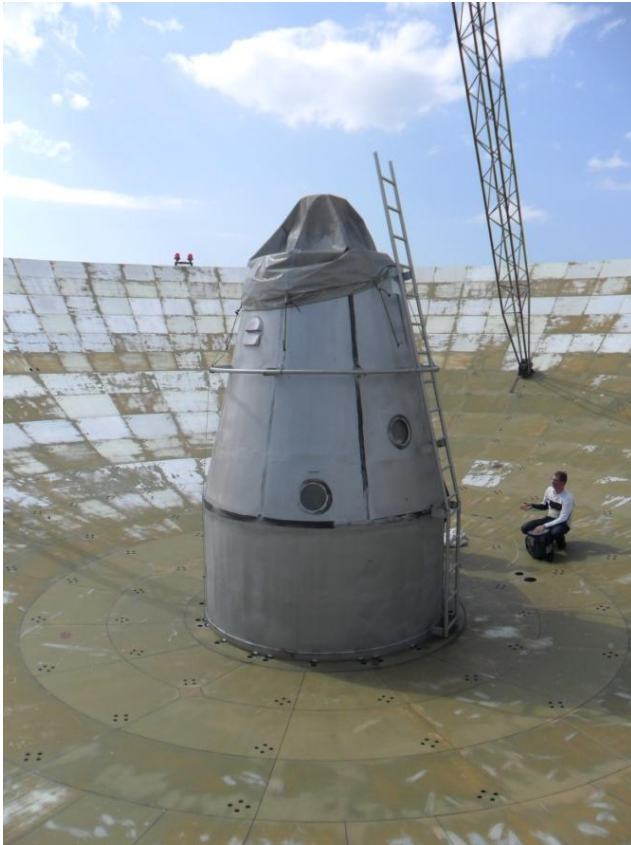
Figure 6 ~ Inside the 32 m dish with a view of the secondary focus. This cabinet will later contain the horn feeds and the cryo-cooled receivers. Colleague Vladislavs is discussing RFI issues with other colleagues inside the enclosure. The RFI level at the secondary focus is much lower than on the prime focus because the deep dish acts like a shield against terrestrial RFI.
